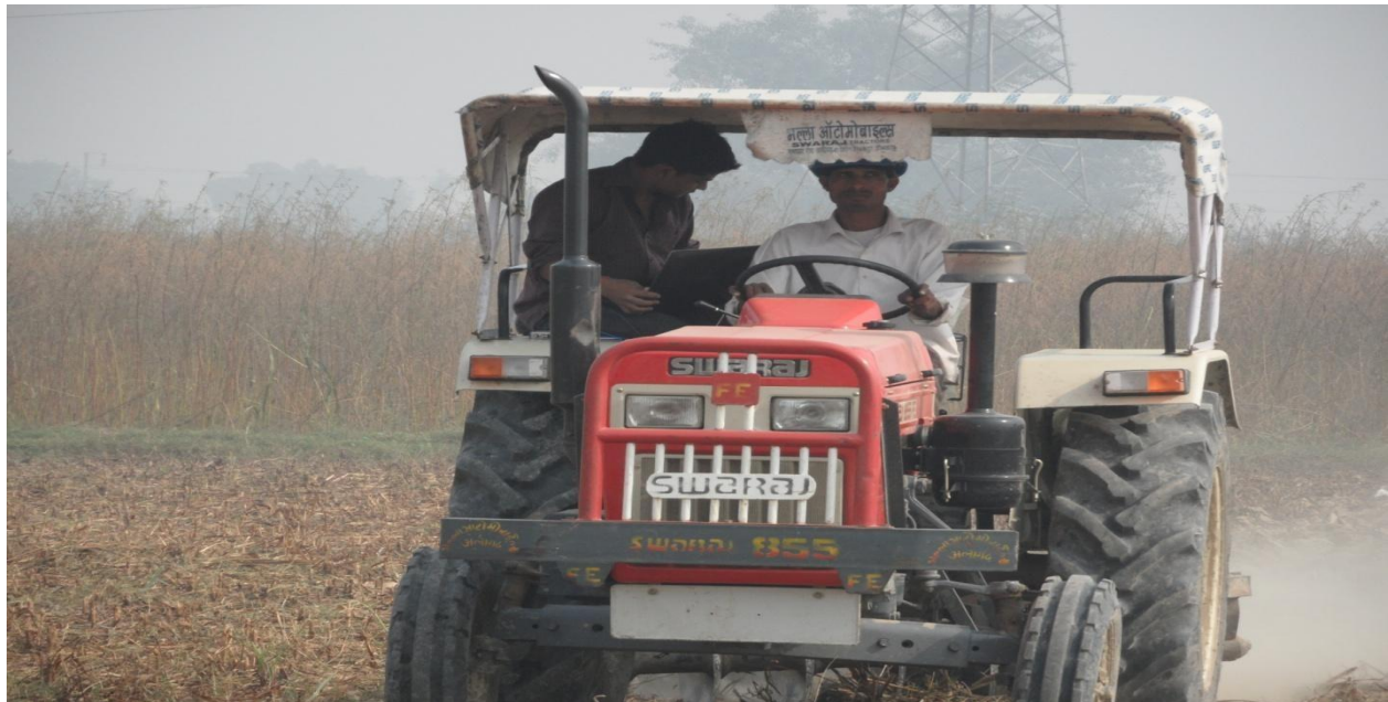
Fig 2: The measurement of vibration of Swaraj tractor 855 FE while harrowing operation.
